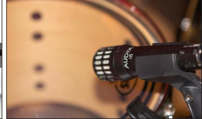
presence to the toms. Note that the i5 is cardioid while the D2 and D4 are hypercardioid. This makes the i5 in theory more prone to bleed from other kit pieces, but I never found that to cause any actual problems when recording or mixing.
